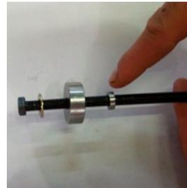
**2 LINKAGE ASSEMBLY** Place two of the dogbone bearings (300020029) and the 1.38" steel pin onto the threaded bolt as shown. Now put on the linkage tool washer and nut (200020071). At this point tighten down the assembly with two 1/2 inch wrenches.
