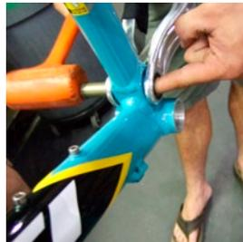
**13 FRAME ASSEMBLY** Install the black washer and button head bolt over the main pivot pin as shown. Cinch the button head down with a 5mm allen key while holding the main pivot with 6mm allen key.
