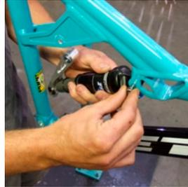
**10 FRAME ASSEMBLY** Thread the male Yeti bolts into the 22mm female bolts and tighten down with 5mm allen keys.
