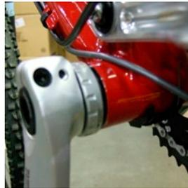
The cable runs parallel along the drive side of the down tube and then slides into the cable guide under the bottom bracket shell. Sometimes the plastic guide from the front derailleur is oriented incorrectly. The cable should run thru the long guide. This should be positioned on the drive side of the bike closest to the crank. Make sure cable does not make contact with frame.
