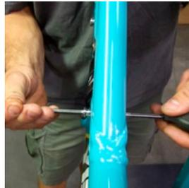
**11 FRAME ASSEMBLY** First slide the swing arm over the main pivot as shown, notice the recess cut in the swing arm in front of the bearings. The recess should be lined up over the main pivot lip to ease the installation process. Slide the seatstays over the steel pivot pin. Now slide the 41.2mm female Yeti bolt and washer through the seatstays and shock assembly. Place a male Yeti bolt with a washer on the non-drive side of the bike. Tighten down both Yeti bolts with 5mm allen keys.
