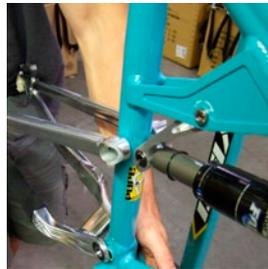
**3 FRAME DISASSEMBLY** To remove the shock mounting bolts, place a 5mm allen key on both ends of the bolts and turn counter-clockwise. Once the male Yeti bolt is removed, take a 6mm allen key and tap out the female end.
