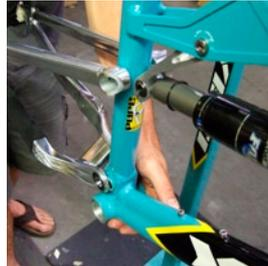
**12 FRAME ASSEMBLY** Make sure the bearings are lined up with the main pivot before tapping the lightly greased main pivot pin through the frame with the dead blow hammer.
