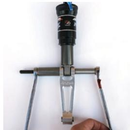
**5 FRAME DISASSEMBLY** Slide a washer and removal slug onto the threaded bolt. Slide this subassembly through the shock and dogbone. On the opposite end, slide on the catch sleeve, washer and then thread the nut on.
