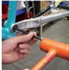
**2 FRAME DISASSEMBLY** Now remove the male and female Yeti bolts that attach the seatstays to the shock and dogbone. You will need two 5mm allen keys in order to back off these bolts. Your swing arm should now be free to slide off the front triangle.
