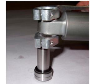
**6 LINKAGE ASSEMBLY** Once you have the pin subassembly started into the shock eyelet, you can slide the threaded bolt, press-cup and press-cup insert configuration from step one through the steel pin subassembly and shock. On the opposite end of the bolt, slide a second nylon washer, the remaining two bearings, press-cup insert, press-cup, washer and nut.
