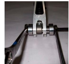
**8 LINKAGE ASSEMBLY** Insert the small socket head cap screws (300030056) into the dogbone and torque down with a 2.5mm allen key. Make sure to prep the bolts with Loctite.
