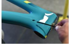
Push the housing into the frame starting at the head tube port until it reaches the bend at the seat tube (you will feel it start to get more difficult to push).
