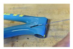
Pull router tool back through the frame until your housing exits the head tube.
