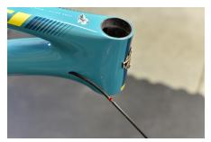
**03.** At the same time, pull the shifter housing out of the head tube port while pushing the seatpost housing into the seat tube until the double barb exits the head tube.
