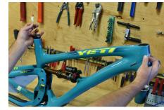
**02.**Pull the Park Tool router through the frame with the clear tubing.
