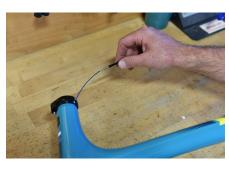
At the seat tube, connect your seatpost housing to the router tool.
