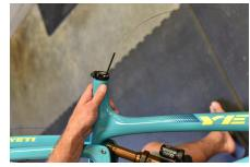
**04.** At the same time, pull the cable up the seat tube while pushing the housing into the head tube port until the housing is fully routed.
