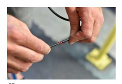
Connect the double-barb to the shifter housing and seatpost housing at the seat tube
