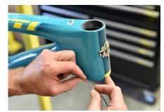
**01.** Remove the lower cable port access cover with a 3mm allen key.
