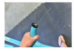
**03.** Leaving the housing stationary, push the cable through the housing until it exits the seat tube.
