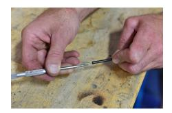
Use a pick to make sure that the inner sleeve of the housing is not crimped
