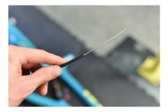
**01.**Install a shifter cable through the seatpost housing, keeping the free end still within the housing.
