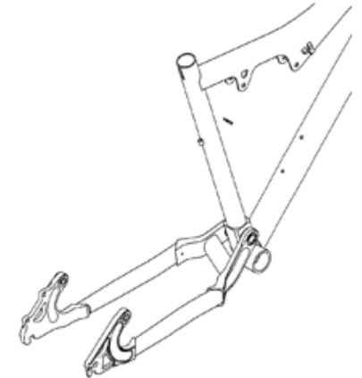
**Figure 5b: Chainstay (5) and ASR Front Triangle (1) with main bearings (7), button head bolts (19), and flat washers (12), assembled**
