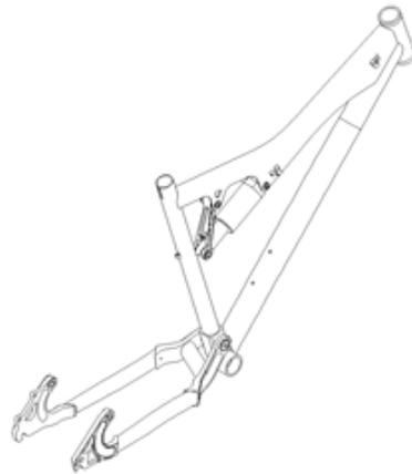
Figure 6b: Dogbone-shock (2-3) assembly mounted to front triangle (1), assembled
