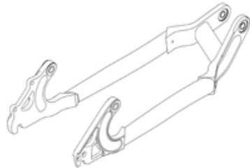
**Figure 4b: Chainstay (5) assembled with main pivot bearings (7), rear pivot bushings (22) and rear bushing inserts(23), assembled**
