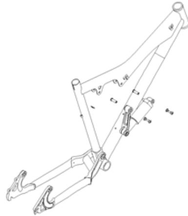
Figure 6a: Dogbone-shock (2-3) assembly mounted to front triangle (1), exploded
