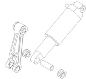
Figure 3a: Dogbone (2) and Shock (3) Assembly with Fox Pin (10) and Black Nylon Washers (11), exploded
