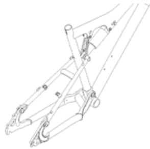
**26 FINAL ASSEMBLY** Put a dab of Loc-tite onto the threads of a button head (19) and insert the button head (19) and washer (12) into the outboard side of the lower seat stay (4). Thread button head (19) and washer (12) into bolt and tighten to 115 in/lbs with a 5mm allen key. Use a second 5mm allen key to hold the sleeve bolt (17) if necessary. Repeat process for other side of seat stay (4).
