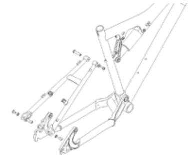
Figure 7a: Attached seatstay (4) to front triangle (1), exploded
