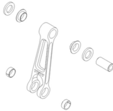
Figure 2a: Dogbone (2) with bushings (22 & 9) and insert (8), exploded
