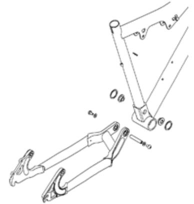
**Figure 5a: Chainstay (5) and ASR Front Triangle (1) with main bearings (7), button head bolts (19), and flat washers (12), exploded**
