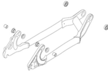
**Figure 4a: Chainstay (5) assemble with main pivot bearings (7), rear pivot bushings (22) and rear bushing inserts (23), exploded**
