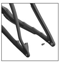
**07**Apply Blue Loctite 243 to threads of the Hanger Stop Bolt (2.5).
