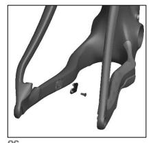
Install the Chainstay Cable Port Cover (2.7) to the non-drive side chainstay port and secure with Flat Head M4 x 10L.
