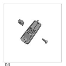
Assemble a Lower Port Clamp (2.15) to the Down Tube Port Cover (2.14) using a Flat Head M4 x 16L screw. Hardware can be torqued to **2-3 Nm** after housing installation.
