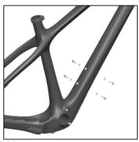
**01.** Grease 4x H20 Bolts (2.2) and install with washers (2.1) to frame downtube.
