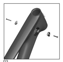
Place a Double Port Clamp (2.12) into the non-drive side cover and a Single Port Clamp (2.11) into the drive-side cover. Secure with M4 x 25L screws.
