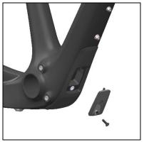
**05**Install the Down Tube Port Cover (2.14) into the frame with a Flat Head M4 x 16L screw (2.16).
