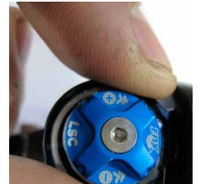
**6 HIGH SPEED COMPRESSION** The HSC adjuster has a twelve click range that can be adjusted by inserting a 2.5mm allen key into one of the angled holes. The HSC adjuster mainly affects the compression damping during medium-to-fast suspension movements.
