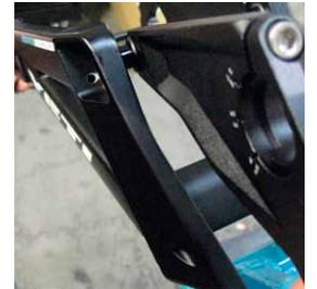
**7 MAIN ASSEMBLY** Rotate each of the push links towards the front of the frame and align the bearing in the link with the pivot pin on the car mount. Flex the link over the pivot pin on the car and tap into place with a dead blow hammer.
