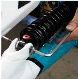
**12 MAIN ASSEMBLY** Install a locktite prepped M6x1x12 Ti male bolt into a 57.5 Ti stud. Slide a 8.5x12.5x.05mm washer onto the stud so that it is flush with the head of the Ti male bolt.
