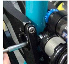
**14 MAIN ASSEMBLY** Using a dead blow hammer push the 57.5 bolt through the eccentrics and shock. Use two 5mm allen keys to tighten the shock with a M6x1x12 Ti male bolt prepped with locktite.
