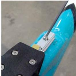
**3 MAIN ASSEMBLY** Slide the swingarm over the main pivot, using the grooves in the swingarm to properly align over the bore.
