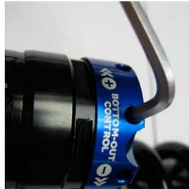
**2 BOOST VALVE** The DHX RC4 has an air pressure range of 125-200 psi, and it must be pressurized. The boost valve allows for seamless transition from small bumps to big drop bottom-outs.
