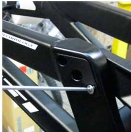
**10 MAIN ASSEMBLY** Slide the front of the shock into the frame mount. Attach the shock to the frame with a M6 x 31mm Ti female bolt and a M6x1x12 Ti male bolt. Use the guide pin tool to align the shock in the frame while inserting the female bolt.
