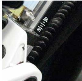
**4 LOW SPEED COMPRESSION** The LSC adjuster has an 18 click range of adjustment that is able to be adjusted by hand. The LSC adjuster primarily affects the compression damping during slow speed suspension movements.
