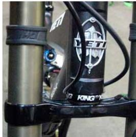
**2 REAR BRAKE** The rear brake line loops across the head tube and into the bolt-on cable stops on the down tube. Use the position closest to the non-drive side on the cable guides for the rear brake line.
