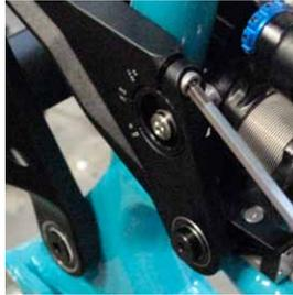
**2 ECCENTRIC ADJUSTMENT** Place a 5mm allen key into each eccentric insert as shown. Rotate the eccentric to the desired position. The eccentric adjustment has a range of 64° / 13.85" – 65° / 14.35".
