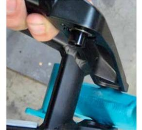
**6 MAIN ASSEMBLY** Press a push link onto each of the exposed pivot pins in the seatstays. Orient the link so that the pinch bolt is facing towards the front of the frame. Note that the links are drive and non-drive side specific.
