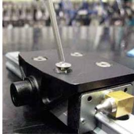
**2 MAIN ASSEMBLY** Attach the rail sub assembly to the frame with three 4x.7x16mm socket head bolts. Prep the bolt threads with locktite. Tighten the bolts using a 3mm allen key. Torque: 40in/lbs
