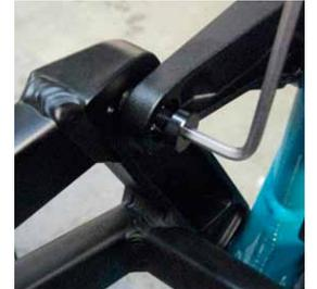
**8 MAIN ASSEMBLY** Tighten four male 12.7mm x 12 mm pivot pin caps into the female pivots pins on the push links and car mount. Prep the male threads with grease. Torque: 65-70in/lbs. At this point the rear triangle will be able to move freely on the rail system. Ensure the car does not dent the seat tube.
