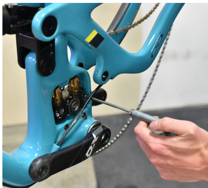
04. Using a needle-type grease gun, push new grease into the two Switch Infinity grease ports until you see grease extruding from the shaft seals.
