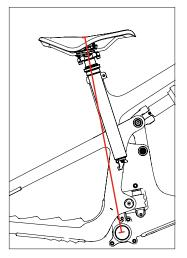
\*These measurements are only for cabled droppers. Please make sure if you have a wireless post you confirm that there is not any interference of the tire hitting the battery when the post is fully dropped and the suspension is fully compressed.
