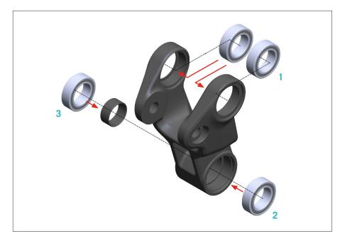
1 Press both upper bearings into the link from the inside of the link tabs using a 15x24mm arbor. Check that both bearings are fully seated.
