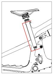
\*Subtract 34mm for a cabled dropper to accommodate housing bend angle.
