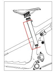
\*Subtract 34mm for a cabled dropper to accommodate housing bend angle.
