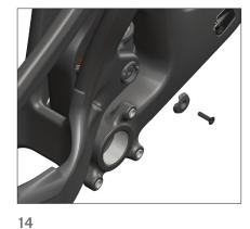
Install Housing Clamp Cap (3.8) onto the driveside main pivot axle with a M4 x 16L FHCS (3.25)
