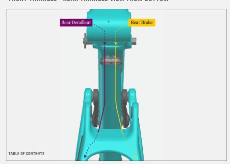
**01** Route brake cable first through the nondrive side port in the rear tri, cable routing grommet, and the top port in the headtube.
