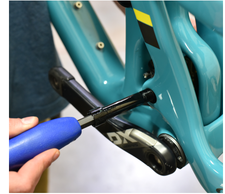
06. Lower the swingarm and re-install your Main Pivot Collet Bolt
