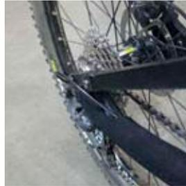
Next route the housing over the bottom bracket and through the cable guide on the front derailleur mount. Run the housing through the two guides on top of the drive side chainstay and affix with cable clips or zip ties. The kevlar chainstay protector should cover the full length housing on the chainstay. Loop the housing into the rear derailleur to finish.
