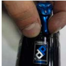
The pro pedal knob has three different levels of dampening: (1) light, (2) medium and (3) heavy pro-pedal. If the bike feels too firm, put it on a light setting, and if it feels too sluggish, turn it to the stiffer setting.
