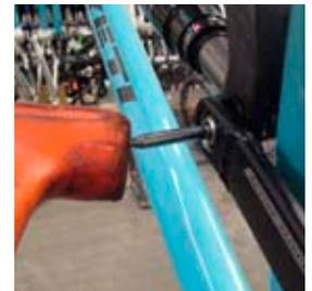
**3 REAR TRIANGLE DISSASSEMBLY** Remove the male main pivot bolt from the female main pivot pin with a 5mm allen key. Use a punch and a dead blow hammer to remove the main pivot pin from the chainstay and front triangle.
