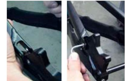
**8 MOUNTING REAR TRIANGLE** Align the top of the seatstay with the bottom of the dogbone and insert the seatstay dogbone pin through the bearings on the seatstays and dogbone on the drive side. Ensure the collar on the pin sits flush with the bearing on the seatstay. Repeat this process for the non drive side of the frame.
