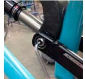
**2 REAR TRIANGLE DISASSEMBLY** Insert the guide pin tool into the stainless female bolt and use a dead blow hammer to tap the bolt out of the frame. Be prepared to catch the bolt as it exits the drive side of the frame. Leave the guide pin in the frame during the next step.
