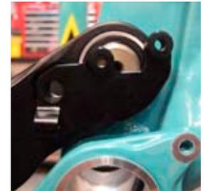
**2 ASR7 FRONT DERAILLEUR MOUNT** Attach the mount with a Ti female M6x16.5 bolt and a M6x1x12 Ti male bolt. Ensure each bolt has the proper washer installed. Prep the male bolt with locktite and tighten the assembly with two 5mm allen keys.
