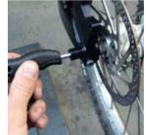
**2 AXLE SYSTEM** Tighten the pinch bolt on the non drive side dropout to secure the axle. Use a 5mm allen key. Torque 75-85 in/lbs
