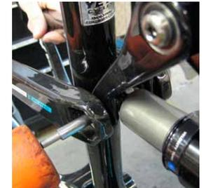
**8 MOUNTING REAR TRIANGLE** Install the main pivot pin (female) from the drive side of the bike. Use a dead blow hammer to push the pin into place. Once the female pivot pin is in place, install and tighten the male pivot bolt with a 5mm allen key. **Torque:**115-125 in/LB
