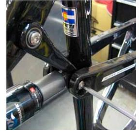
**2 REAR TRIANGLE DISASSEMBLY** Insert the guide pin tool into the 46.5 female bolt and use a dead blow hammer to tap the bolt out of the frame. Be prepared to catch the bolt as it exits the drive side of the frame. Leave the guide pin in the frame during the next step.
