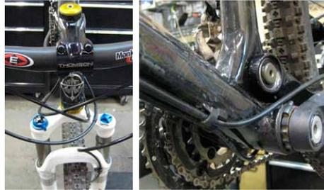
The wire cable will run the length of the down tube, through the guide on the bottom bracket shell, and then attach to the front derailleur.
