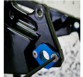
**6 INSTALLING SHIMANO DROPOUT KIT** Insert the M4x6MM custom cap bolt into the top of the drive cap. This bolt will be used to set the position of the Shimano 142x12MM axle. Refer to Shimano literature for exact instructions on axle operations.
