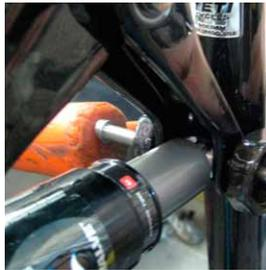
**10 BOTTOM BRACKET INSTALLATION** Apply a thin layer of grease to the inside of the bottom bracket shell. Push the drive side bottom bracket cup into the frame by hand. Ensure the cup is straight and tap flush into the frame with a dead blow hammer. Repeat the process on the non drive side of the frame.
