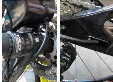
Next route the housing under the bottom bracket and through the drive side chainstay and loop onto the derailleur. Run the housing through the hole on the chainstay and push it through the exit hole by the rear derailleur. Remove the cap on the exit side of the chainstay to make this process easier. Ensure to leave enough "slack" between the last cable stop on the down tube and the chainstay to allow for smooth shifting when the rear suspension is being compressed.
