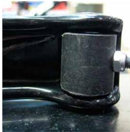
**2 DOG & SHOCK MOUNTING ASSEMBLY** Use a dead blow hammer to install two 23.5mm reducers into the lower portion of the shock.
