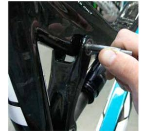
**6 REAR TRIANGLE ASSEMBLY** Slide the swingarm over the main pivot, using the grooves in the swingarm to properly align over the pivot.
