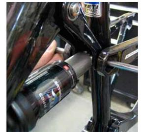
**3 SHOCK & DOGBONE DISASSEMBLY** Remove the male main pivot bolt from the female main pivot pin with a 5mm allen key. Use a punch and a dead blow hammer to remove the main pivot pin from the swingarm and front triangle.
