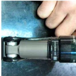
**4 DOG & SHOCK MOUNTING ASSEMBLY** Install the shock and dogbone on the frame. Insert a 34.0 mm Ti female bolt through the drive side of the frame for the shock. Use a Ti male bolt on the non-drive to tighten the shock into place with a 5mm allen key. Support the bottom of the assembly while tightening the shock to the frame. **Torque:**90-95 in/LB
