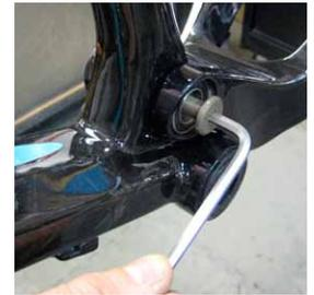
**4 SHOCK & DOGBONE DISASSEMBLY** Remove the guide pin from the seatstay junction and then pull the rear triangle off of the frame. Remove the male bolt from the 40.5mm Ti female bolt holding the dogbone in place. Use the guide pin and a dead blow hammer to tap the female bolt out of the frame.
