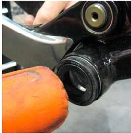
**11 COMPLETE ASSEMBLY** Double check alignment of all frame components and refer to the torque settings chart to ensure all bolts are properly tightened on frame.
