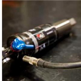
**2 SAG** Once you have set your baseline air pressure you need to measure the sag. To measure the sag slide the travel indicator (O-ring) up against the shock body. Next compress the shock by sitting on your bike and then get off. The distance between the shock body and the new position of the travel indicator (O-ring) is your sag. Refer to the guide below for the % of sag equivalents for the measurement recorded.
