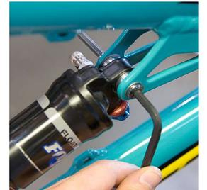
**8 FRAME ASSEMBLY** Secure the main pivot bearings via the pinch bolts. Tighten the Bolt Cap M5 X 0.8 X 24 mm using a 4mm allen key.
