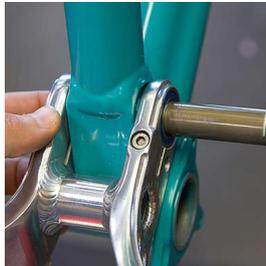
**11 FRAME ASSEMBLY** Tap the pin through the bearings and frame via a dead blow hammer.
