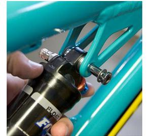
**7 FRAME ASSEMBLY** Thread the Pivot Bolt Male Yeti (M6 X 17 mm) and Washer (8.5 X 12.5 X 0.5 mm) in the female bolt and secure using a Two 5mm allen keys.
