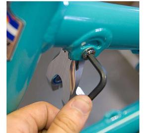
**6 FRAME ASSEMBLY** Place the head of the shock into position on the mounting tabs as shown.
