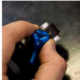
**4 REBOUND** The rebound adjustment has a 9 click range. As a general rule, adjustments that are too fast (counter-clockwise adjustment) will produce a springy ride with excessive kick up of the rear end causing bucking of the rider. Adjustments that are too slow (clockwise adjustment) will cause packing of the rear wheel that is identified by a sluggish ride feeling.
