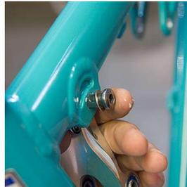
The slide the Pivot Bolt Female Yeti (M6 X 24.8 mm) and Washer (8.5 X 12.5 X 0.5 mm) through the frame and Dogbone as shown.
