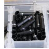
**HOUSING END CAPS** Yeti recommends using metal end caps. The metal caps do not allow the cable to pull through as do the plastic versions. Do not mix up the shift and brake housing because it will result in a loss in performance.
