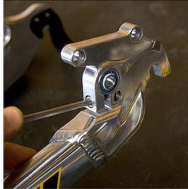
**10 FRAME ASSEMBLY** Slide the swingarm assembly into position on the frame as shown. Make sure to line up the inner race of the bearings with the thru-hole on the frame.
