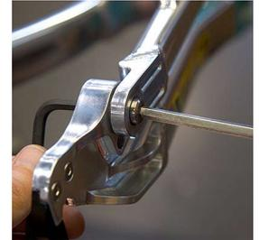
**12 FRAME ASSEMBLY** Before making the final connection thread one the remaining Bolt-Ti-Male (M6 X 1 X 12 mm) and Washer (8.5 X 12.5 X 0.5 mm) into the Stud-Ti-Female (M6 X 8 X 53 mm). Just secure finger tight. The purpose is to create a bolt sub-assembly for the final connection.
