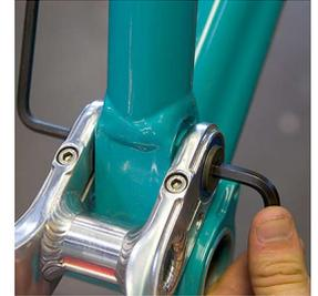
**14 FRAME ASSEMBLY** Place the seatstays onto the chainstay assembly. Line up the thru-holes on the seatstay with the inner race of the bearings on the chainstay.
