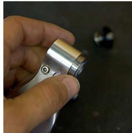
**2 LINKAGE ASSEMBLY** Once both bearings and in the proper position secure the bearings via the pinch bolts. Tighten the Bolt Cap M3 X 0.5 X 12 mm using a 3mm allen key.
