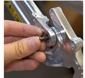
**11 FRAME ASSEMBLY** Secure the male and female bolts using two 5mm allen keys.
