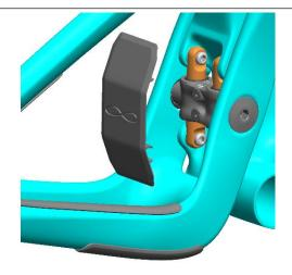
Pull the Switch Infinity Fender from the frame, unclipping it from the Switch Infinity bolt heads. Gently clean the Switch Infinity Link with a rag and mild detergent or alcohol
