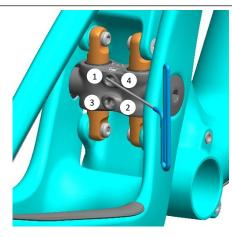
With a 2mm Allen key, back-off the four preload set-screws completely. Gently tighten each screw until it contacts the shaft bushings. Alternating between each shaft, tighten each set screw an additional 1/8 turn to preload the bushing.
