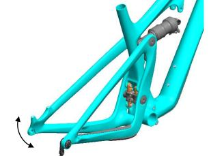
We recommend removing the front shock mount and cycling the suspension to ensure smooth movement. Protect your frame from any shock strikes. If there is any excessive friction within the system, decrease the bushing preload slightly.
