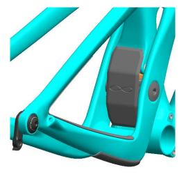
Clip the Fender back onto the frame. Service is now complete.
