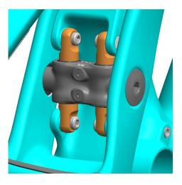
Apply a small drop of Blue Loctite to the Preload Access Screws. Reinstall and torque to 3 Nm.
