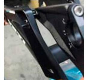
**7 MAIN ASSEMBLY** Rotate each of the push links towards the front of the frame and align the bearing in the link with the pivot pin on the car mount. Flex the link over the pivot pin on the car and tap into place with a dead blow hammer.
