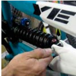
**11 MAIN ASSEMBLY** Ensure the female bolt enters the frame through the drive side and that each Ti bolt has the appropriate washer. Apply locktite to the male bolt and tighten using two 5mm allen keys.
