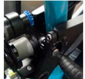
**15 MAIN ASSEMBLY** Adjust the eccentrics to the desired position and secure the pinch bolts on the push links using a 5mm allen key.
