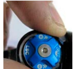
**6 HIGH SPEED COMPRESSION** The HSC adjuster has a twelve click range that can be adjusted by inserting a 2.5mm allen key into one of the angled holes. The HSC adjuster mainly affects the compression damping during medium-to-fast suspension movements.
