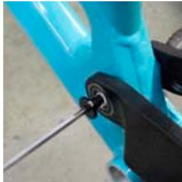
**5 MAIN ASSEMBLY** Press a 12.7mm x 18mm pivot pin through each of the bearings located at the top of the seat stays on the rear triangle. Orient the pin so the exposed female threads are on the inside of the seatstays.
