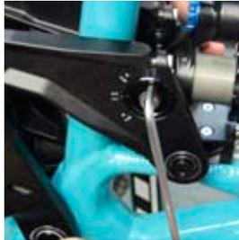
**3 ECCENTRIC ADJUSTMENT** Once the eccentric mount is in the preferred position secure the pinch bolts.
