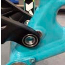
**4 MAIN ASSEMBLY** Install the main pivot pin from the drive side using a dead blow hammer. Be sure to lightly coat the pivot pin with grease. Thread the main pivot pin cap into the non drive side of the pivot pin. Use a generous amount of grease on the male threads. Tighten the pin and cap with two 5mm allen keys. Torque 100 in/lbs
