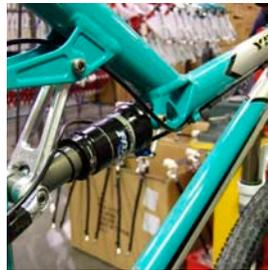
**3 REAR BRAKE** Run the brake line across the head tube to the first open cable drop out on the non-drive side of the top tube.
