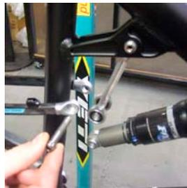
**3 FRAME DISASSEMBLY** To remove the shock mounting bolts, place a 5mm allen key on both ends of the bolts and turn counter-clockwise. Once the male bolt is removed, take a 6mm allen key and tap out the female end.
