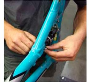
**6 FRAME ASSEMBLY** First slide the swing arm over the main pivot as shown. Notice the recess cut in the swing arm in front of the bearings. This recess should be lined up over the main pivot lip to ease the installation process. Place the plastic washers on both sides of the steel pin as shown. While holding the washers in place slide the seatstays over the washers and dogbone.
