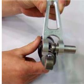
**2 LINKAGE ASSEMBLY** Slide a washer of the linkage tool (200020071) on the threaded bolt then slide this through the removal slug (1.5" long). Then slide on the shock pin. Slide the tool assembly through the dogbone and shock eyelet. On the opposite side slide on the catch sleeve and washer, and then the nut. Place the wrenches on the tool assembly and tighten, installing the shock pin.
