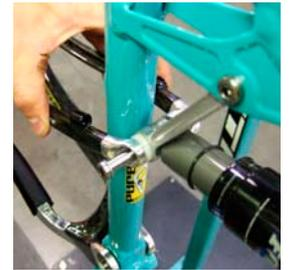
**8 FRAME ASSEMBLY** Make sure the bearings are lined up with the main pivot before tapping the lightly greased main pivot pin through the frame with the dead blow hammer.
