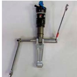
**3 LINKAGE ASSEMBLY** While turning the tool make sure you press the shock pin into the correct position. The easiest way to gauge this is to use one of the white nylon washers. The relief on the pin should be even with the washer.
