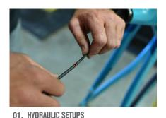
Route a section of shifter housing through the frame using the steps described in Standard Setups. Connect the double-barb to the shifter housing and the seatpost housing at the seat tube.
