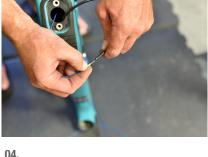
Outside of the access port, connect the Park router tool to the housing.
