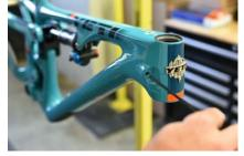
**02.**Install your seatpost housing into the head tube port, pushing until it exits near the lower cable port access hole.
