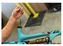
Pull router tool back through the frame until your housing exits the seat tube.
