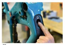
Use your finger to help push the housing around the bend in the frame up into the seat tube.
