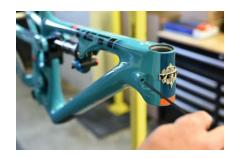
Push your seatpost housing into the frame from the headtube port until it exits near the access port.
