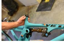
While pushing the housing into the head tube port, continue pushing the cable up the seat tube through the access port until the housing exits the seat tube.
