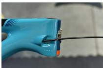
At the same time, pull the shifter housing out of the head tube port while pushing the seatpost housing into the seat tube until the double barb exits the head tube.
