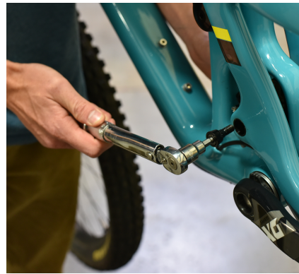
07. Install the Main Pivot Collet Wedge and *Torque to 14 Nm.
