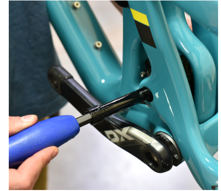
06. Lower the swingarm and re-install your Main Pivot Collet Bolt prepped with Blue 243 Lcotite.
