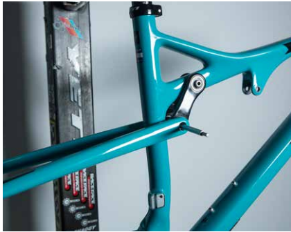
13. Use a Fox guide pin to align the link, spacers and the swingarm.
