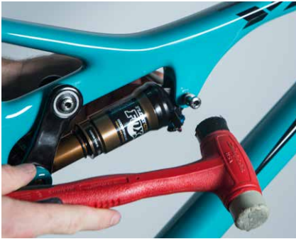
17. Using the guide pin slide the front shock mounting hardware through the frame and shock. Use a soft mallet to tap it through if necessary.
