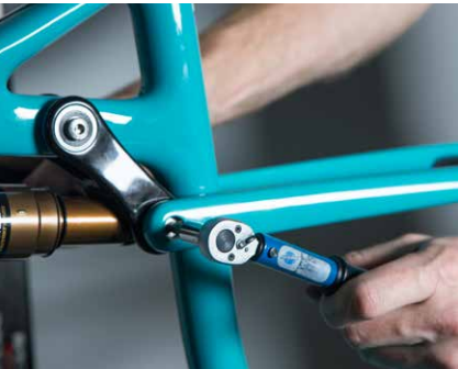
19. Using a well calibrated torque, wrench tighten the lower link hardware to 6.5 Nm. Torque to 6.5 Nm
