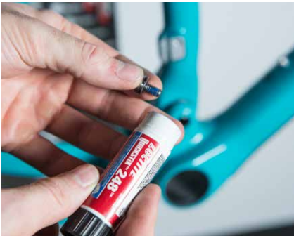
18. Apply blue (248) Loctite to the male bolts for the shock mount and the lower link pivot at this time.
