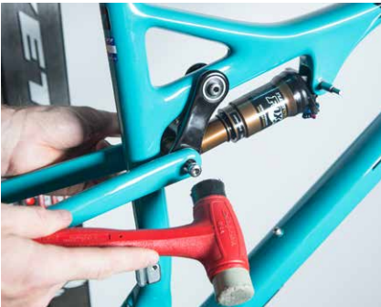
16. Using the guide pin, slide the lower link pivot hardware through the swingarm, link and shock. Use a soft mallet to tap it through if necessary.
