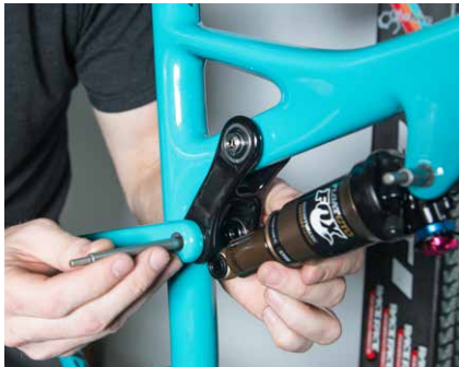
15. pull the lower link guide pin back, leaving it partially in place. Give yourself clearance for the rear of the shock to slide into place. Place the shock into the link and reinsert the guide pin.
