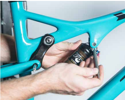
14. Slip the front shock mount into the front triangle and use another Fox guide pin to align and hold it in place.
