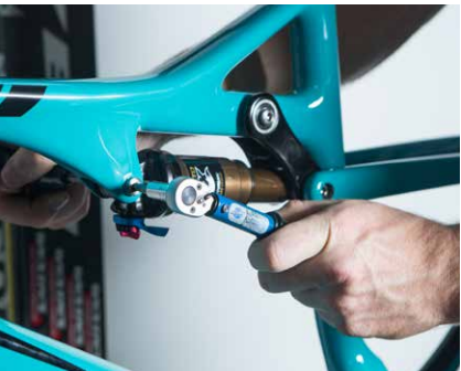
20. Using a well calibrated torque, wrench tighten the front shock mounting hardware to 6.5 Nm. Torque to 6.5 Nm
