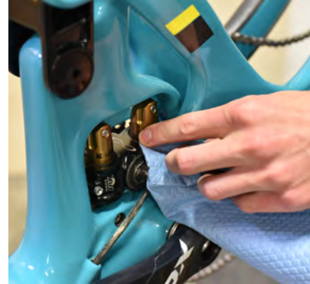
05. Wipe off any excess grease that was pushed out of the seals.
