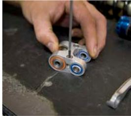
**2 LINKAGE ASSEMBLY** Slide the u-shaped end of the Shortlink over the back end of the shock. Make sure you slide the Shortlink over the proper end of the shock with the rebound knob facing down and the pinch bolts facing up.
