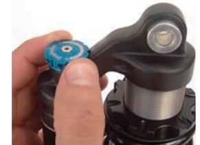
**4 SAG SETUP** Use 25-35% of the shocks stoke for trail riding/freeride use and 30-40% for downhill use. To determine sag, first measure the distance between the centers of each shock mounting bolt (eye-to-eye) and record this number. Make sure you have the correct spring for your weight. See the spring rate chart.
