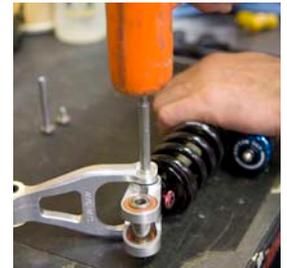
**6 LINKAGE ASSEMBLY** Thread the Button Head Bolt (M6 X 1 X 12 mm) onto the Bolt-Ti-Stud (M6 X 53 mm). Make sure to use a small amount of blue Loctite on the threads. The slide one Washer (8.5 X 12.5 X 0.5 mm) onto the bolt and stud assembly.
