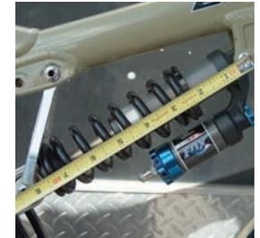
**5 SAG SETUP** Next, sit on the bike and record the new (eye-to-eye) measurement. Subtract the static eye-to-eye measurement from this new measurement and you get your sag in inches. An easy way to calculate sag is to multiply the shock travel by your desired sag percentage.
