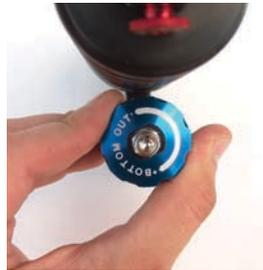
**Warning:** When the volume adjuster has reached its counter-clockwise stop limit, continued force on the adjuster may cause damage to the adjuster mechanism.
