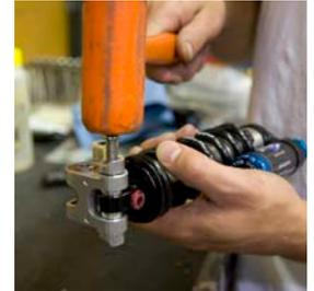
**8 LINKAGE ASSEMBLY** Thread the Button Head Bolt (M6 X 1 X 12 mm) on the other end of the Ti-Stud. Once again make sure to apply a small amount of blue Loctite.
