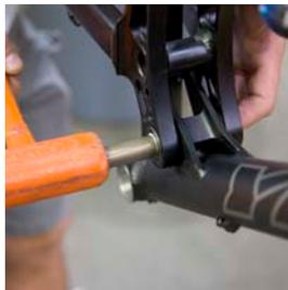
Slide the Main Pivot Pin (M6 X 17 X 67.5 mm) into the bearing and tap through the frame with a dead blow hammer. There may be some resistance as you tap the pin through, this is normal. Tap the pin until it sits flush against the bearing face,
