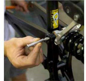
Slide the Washer (8.5 X 12.5 X 0.5 mm) onto the Female Yeti Bolt 43mm. Then attach the bolt and washer to the stepped end of the Guide Pin.
