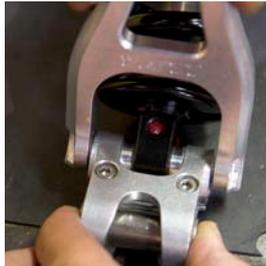
**4 LINKAGE ASSEMBLY** If necessary use the Yeti Guide Pin to line up the Dogbone, Shortlink and shock eyelets by sliding the Guide Pin through the sub assembly.
